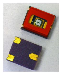
Marktech Optoelectronics has just released its new line of Avalanche Photo Detectors (APD) in Surface Mount Packages. These devices are available in two optimized wavelengths—800nm and 905nm—and are now available at Digi-key.com. Featuring a choice of a circular 0.04 or 0.2mm² active area and housed in a LCC3 or LCC6 SMD package, they are well-suited for applications requiring high speed and low noise in visible-near IR applications such as time of flight measurements (Lidar).
